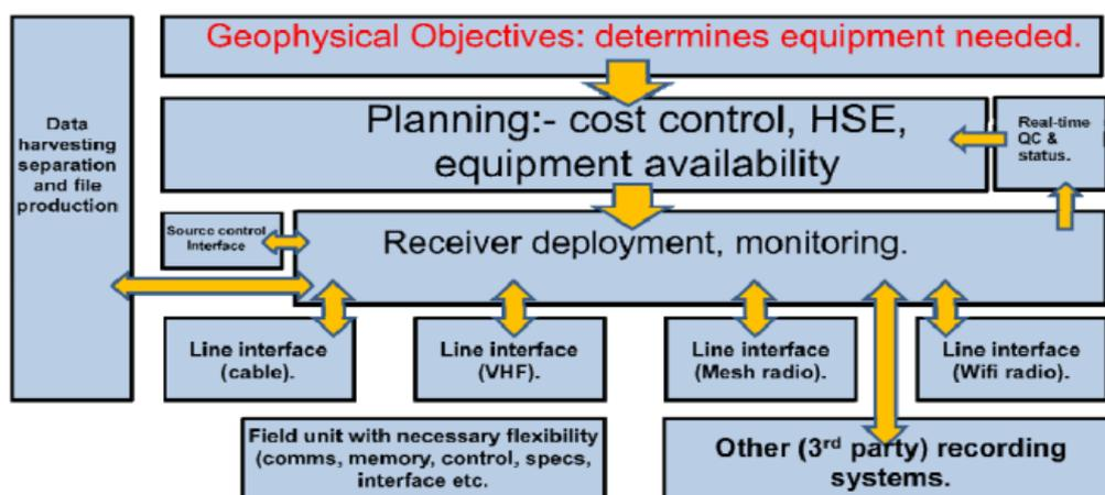
Figure 1. General purpose recording system architecture suited to wavefield recording.
