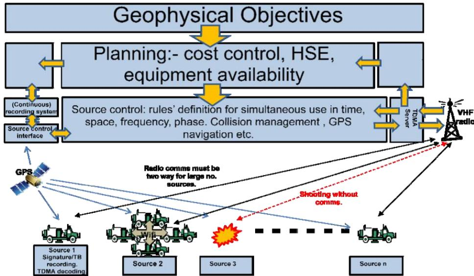
Figure 2: General purpose source control system architecture suited to wavefield recording.
