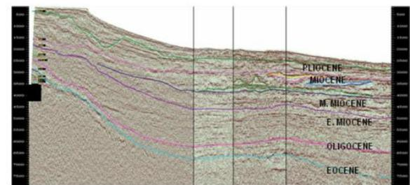
FIG 4 Regional 2D line passing through study area showing channel levee system
