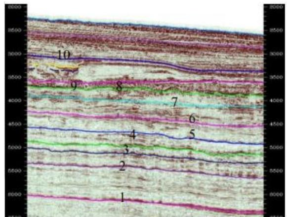
Fig 5 Seismic trace showing mapped levels in the study area
