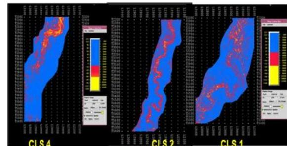
Fig.10: Average absolute amplitude between Ref10(PS 4) & Ref 9 showing high amplitude along channel (CLS 4) between Reflector 8a (PS 5) & 8 (PS 2) showing high amplitude with CLS 2 between PS 2 & 3 of Reflector 4 showing high amplitude within CLS 1
