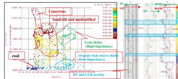
Fig. 6 Cross-plot between impedance and gamma-ray log for an interval consisting of source rock, shale, coal, sand/silt and carbonate in a well from Western Offshore Basin. Source intervals are identified by high gamma and neutron porosity, relatively high resistivity, and very low velocity and density.
