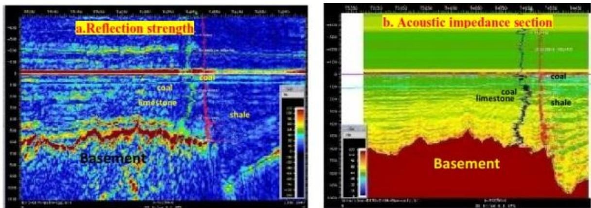
Fig. 5 Reflections strength and impedance sections showing signature of shale layers. a. amplitude section. b. Impedance section. Intercalated shale layers can be mapped by impedance.
