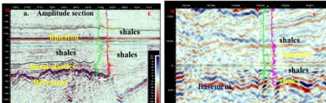
Fig. 3 Seismic sections showing signature of shale layers. a. Thick shales with thin coal, limestone, silt etc. b. Thin shales interbedded with coal, limestone, sandstone etc. Both sections are flattened at upper sequence boundary (Lower Eocene)
