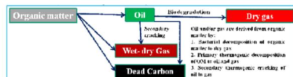
Fig. 1 Schematic showing decomposition of Organic matter in Oil and Gas
