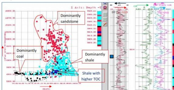
Fig. 2 Cross-plot between Gamma-ray and acoustic impedance showing properties of shaly intervals with respect to coals and sandstones, in a well from Upper Assam Shelf Basin. Points are colour-coded with respect to lithology. Shaly intervals are identified by high gamma and low impedance. Shales with higher TOC are identified from sonic-resistivity overlay.
