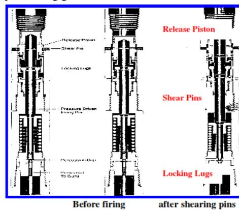
The advantage of this firing method is that, after setting the packer, the tubing and packer can be tested in the direction of well pressure by internally pressurizing the tubing and transmitting this pressure to casing, beneath the packer.
