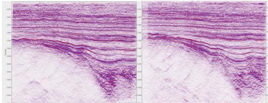
Substantial improvement in the standout of deeper reflections over Diu arch has given an impetus to redefine the Mesozoic sequences and given a ray of hope to reinterpret the area and explore the hydrocarbon potential for the Mesozoics deposited over Diu arch and re-orient drilling objective accordingly.
