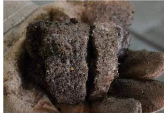
Figure 2 : Frozen sand sample after compression test
