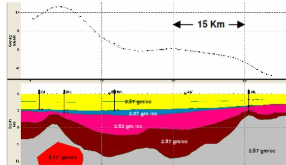
Fig. 6. Residual gravity modeling along profile DD
