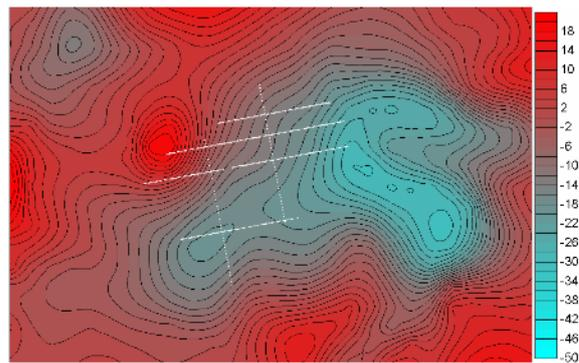
Figure. 4a. Residual gravity map of the study area (60x60 Km) after high pass Gaussian filter of wavelength shorter than 136 Km.
