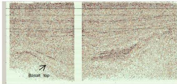
Fig 5 . Seismic section along profile DD/ showing the top of the basalt.
