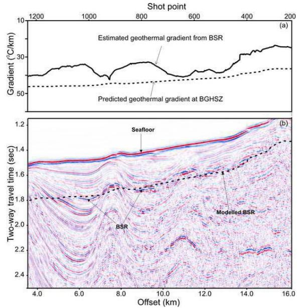
Figure 3: (a) Estimated geothermal gradient (shown with solid curve) from the position of the BSR and the predicted geothermal gradient (dotted curve) at BGHSZ. (b) 2D MCS profile with low amplitude BSR is observed. Modeled BGHSZ (or BSR) is shown with dotted black line.
