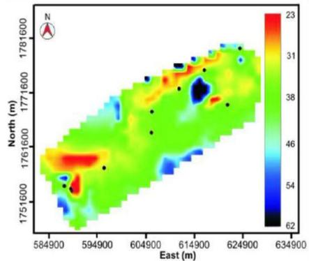
Figure 4: Regional heat flow map derived from the observed BSR depth on 2D seismic section. The color bar represents the heat flow values in  $mW/m^2$ .
