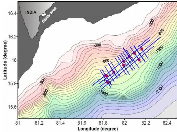
Figure 1: Bathymetry map of the Krishna-Godavari (KG) basin, off the eastern Indian margin. Location of drill sites by the NGHP-01 are shown with red circles. Solid blue lines are the 2D high resolution MCS lines. Bold red lines with corresponding figure numbers represent the lines used in this study. The color bar represents the water depth in meter below seafloor. Contours are also shown to indicate water depth directly. Inset shows location of the KG Basin on the east coast off India.
