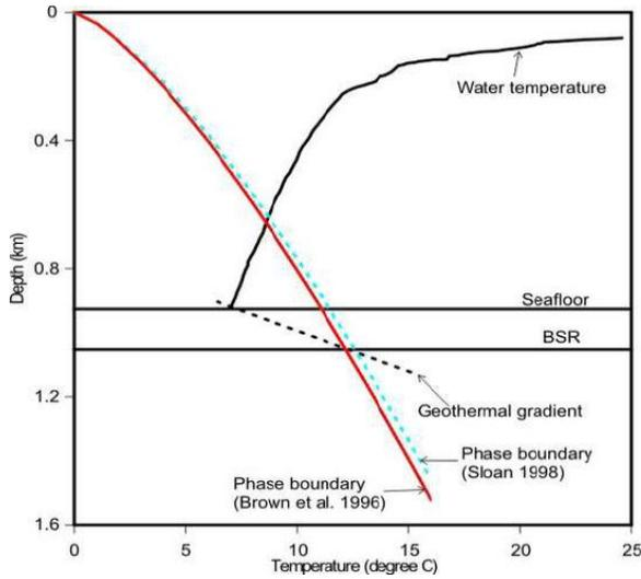
Figure 2: Methane hydrates stability curve of Brown et al. (1996) and Sloan (1998) for site 15 of NGHP-01 in the KG basin. Geothermal gradient interpolated from the in situ temperature measurements. Water temperature profile of CTD measurements is taken from Mazumdar et al. (2007).
