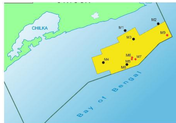
Fig-1 Map showing the area under study (yellow part) with drilled wells (Black dots for dry, Red for gas wells)
