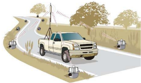
Figure 2: Example of remote data harvesting of Acquisition Units using a mobile Wi-Fi antenna, while acquisition is not discontinued
