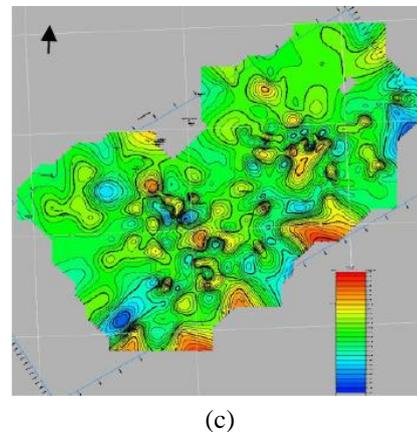
Figure-5: Elevation and thickness contouring of Shallow weathered layers in Namrup-Borhat area, (a) elevation contour of the area, (b) thickness contour for first layer, (c) thickness contour for second layer.
