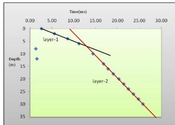
Figure-7: Depth time curve from uphole for Jorajan shows two layers model.
