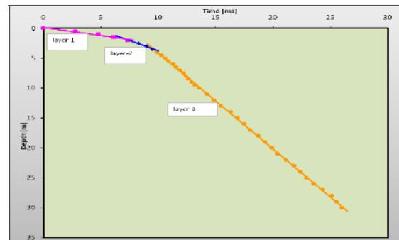
Figure-3: Uphole data indicates three layers model for Amguri area.
