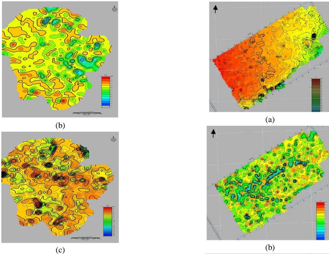
Figure-4: Elevation and thickness contouring of Shallow weathered layers in Amguri area, (a) elevation contour of the area, (b) velocity contour for first layer, (c) velocity contour for second layer.
