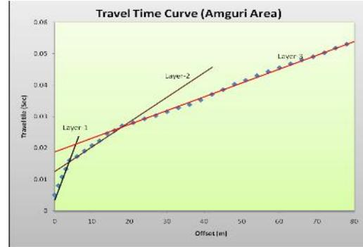
Figure-2: Travel time curve from refraction data for amguri shows three layers model.
