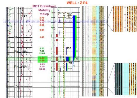
Fig.6 Composite plot of PLT, MDT, FMI and Conventional Log for Well: Z-P4
