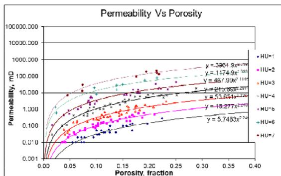
Fig.9 Porosity-Permeability Plot with Hydraulic Unitisation,
