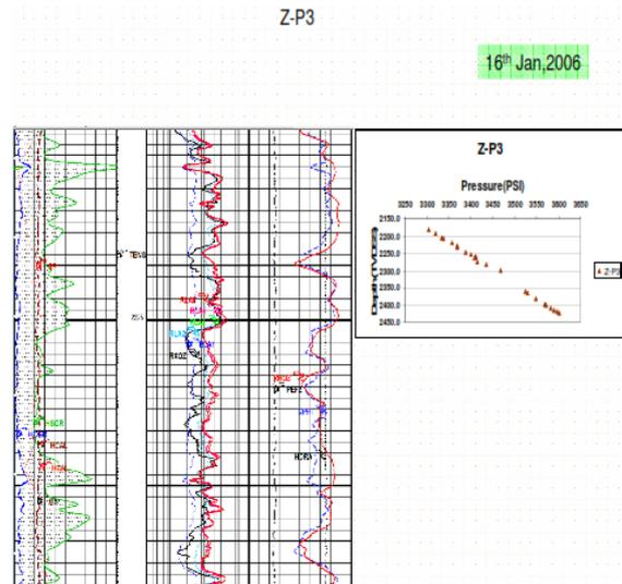
Fig3. Log Profile against Pay-II and MDT Pressure Plot for Well: Z-P3
