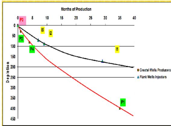
Fig.5 Differential Depletion Trend for Producers and Injectors for Z-Field.
