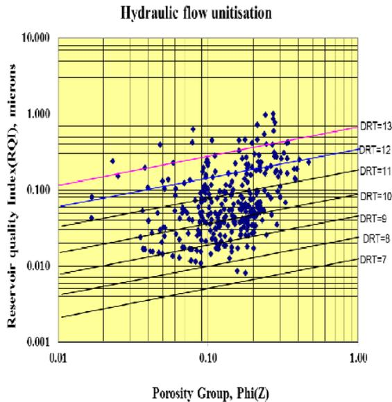
Fig.8 Hydraulic Flow Unitisation through DRT
