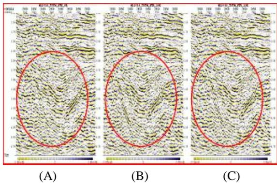
Figure-7: The impact on PSTM Stack for varied migration aperture with full aperture of (A) 8 km; (B) 16 km; and (C) 12 km.
