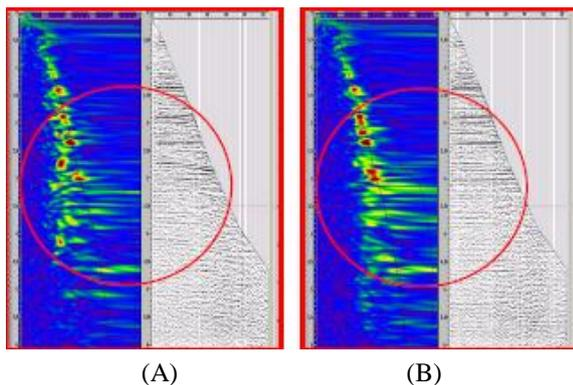
Figure-8: The PSTM Gather output alongwith the semblance plot (A) Before removal of multiples & (B) After removal of multiples.
