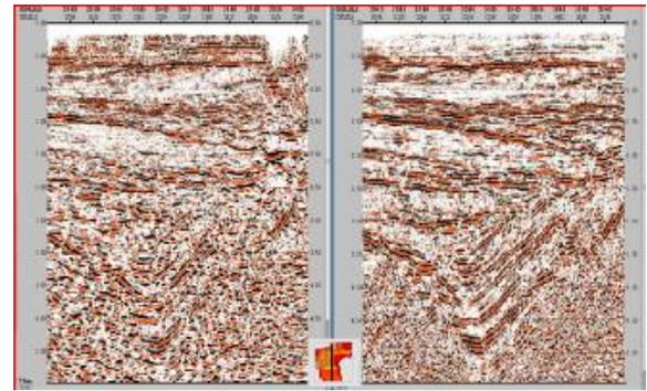
Figure-12: Comparison of PSTM sections of Crossline 3040. (a) Earlier 3D individual volume PSTM Stack and (b) 3D Pre-stack merged volume PSTM Stack.
