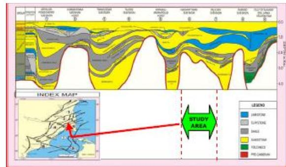
Figure-3: Schematic geological section through different tectonic elements of the Cauvery basin.
