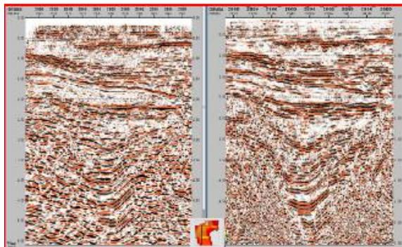
Figure-11: Comparison of PSTM sections of Crossline 2800. (a) Earlier 3D individual volume PSTM Stack and (b) 3D Pre-stack merged volume PSTM Stack.
