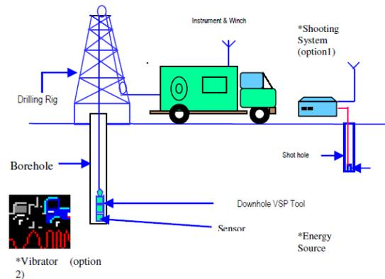
Fig 2: Schematic diagram of VSP's operation
