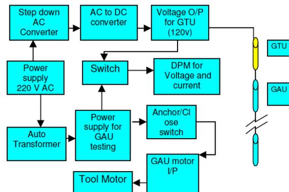
Fig 5: Block Diagram of VSP Tool Test Panel
