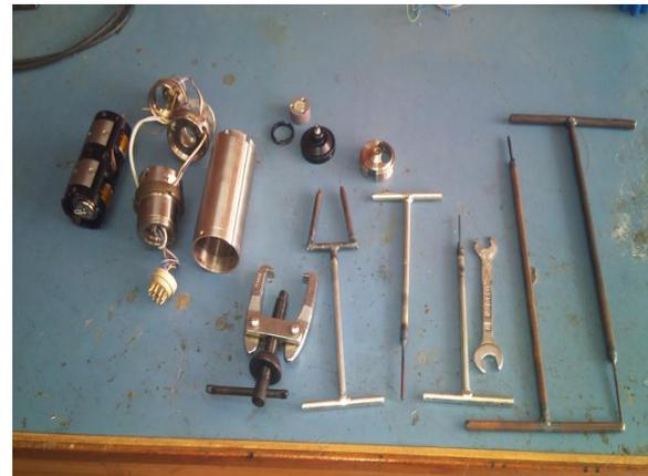
Fig 7: Geophone cartridge along with designed tools
