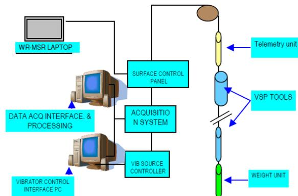
Fig 3: Schematic diagram of multilevel VSP system
