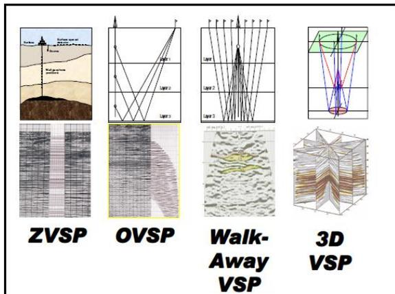
Fig 1: Various types of VSP's and its seismic outputs
