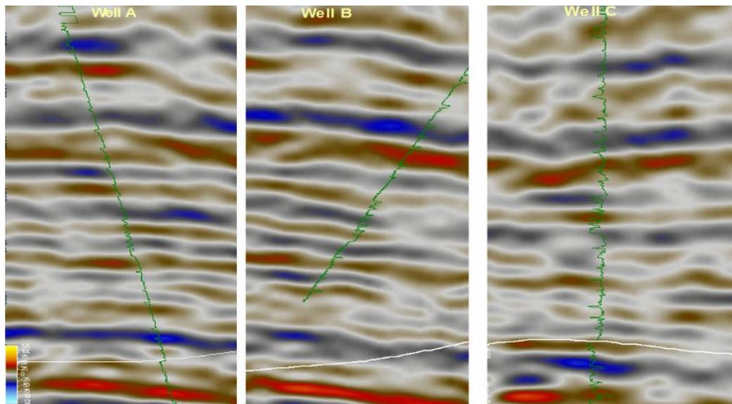
Fig 7: Gamma Log superimposed on PSDM volume. In well B real time data is being streamed.
