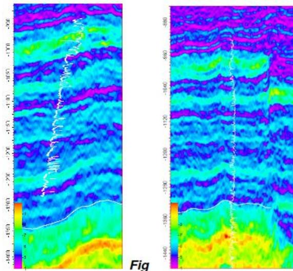
Fig 4: Gamma Log superimposed on inversion volume. In well B real time data streaming
