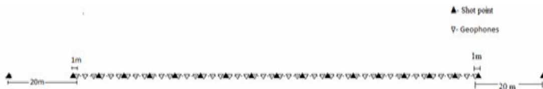
Figure 3: Arrangement of geophones and shot points on a survey line
