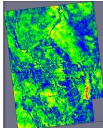
Fig 4. Absolute amplitude attribute map on top of horizon D showing the possible presence of a channel in the north-eastern part of the study area.
