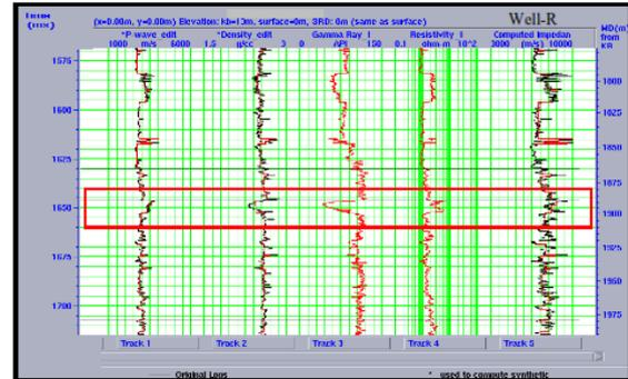
Fig-3: Edited Sonic and Density logs of well R (resampled at 2msec) in track 1 and 2. Zone of interest is marked with red rectangle.
