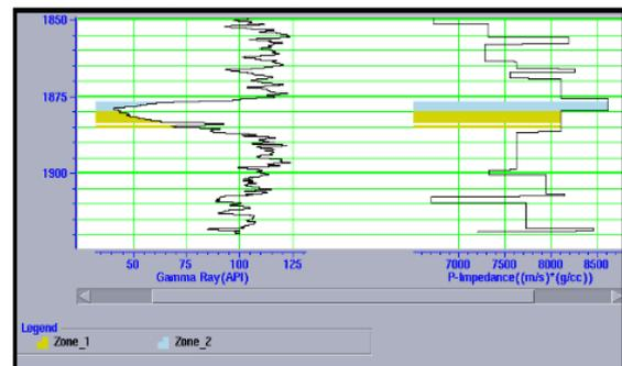
Fig-4b: Vertical cross-section of cross-plot of well R. Reservoir sands are of high impedance compared to nearby shale on top and bottom of pay.
