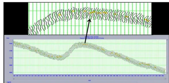
Fig-12 Intercept attribute derived from AVO inversion overlaid with AVO anomaly identified from the intercepts / gradient cross-plot. Zoomed part of the section placed on the top. AVO anomaly is observed at many places on this line which are possible hydrocarbon exploration leads.
