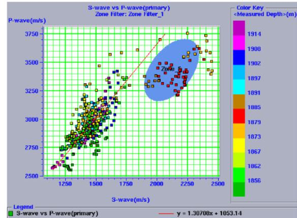
Fig-5: Cross-plot  $V_p$  versus  $V_s$  logs (well R) in the interval 1850-1920m. Data points from gas reservoir sands zone are marked with blue ellipse clearly showing separation from background trend of shale.
