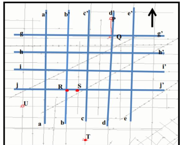
Fig-2: Map showing location of seismic lines and drilled wells. Part of seismic lines re-processed shown in blue color.
