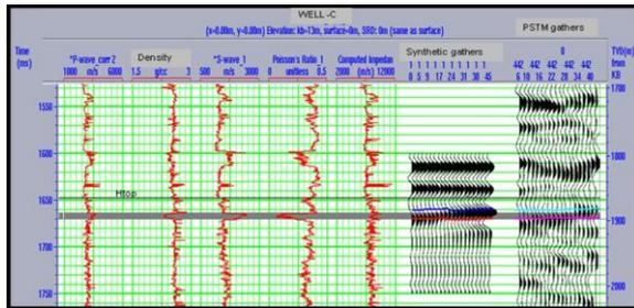
Fig -7 AVO Synthetic model for the In-situ, gas charged sand package to the left and the seismic gathers at well R to the right show phase reversal on far offset traces on the top of reservoir i.e., from Trough to Peak response classified as class II AVO anomaly. Density log shows drop in density due to gas effect but computed impedance is even higher for reservoir zone than background shale. Track 1 to 5 is Sonic, Density, Shear log, computed Poisson's ratio and Impedance log respectively.
