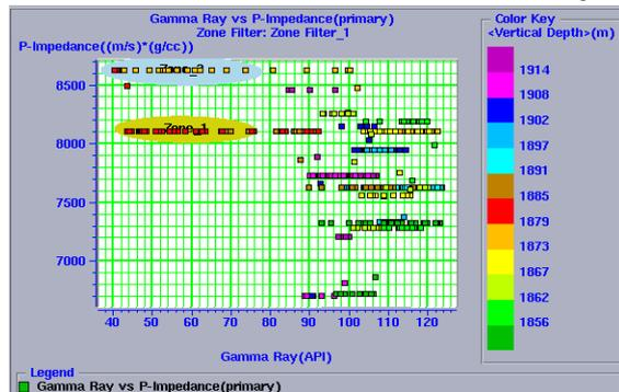
Fig-4a: Cross-plot GR versus computed impedance derived from sonic and density logs for the interval 1850-1920m for well R. Object in the interval 1889 -1898(1876- 85m TVD) flowed gas. Reservoir sand marked with light blue and yellow color has relatively high impedance compared to the shale above and below.
