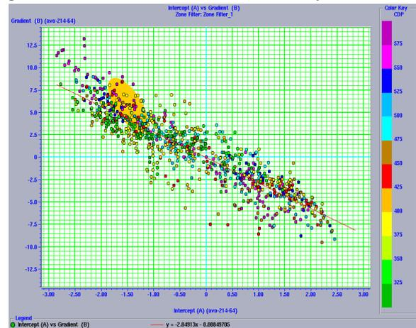
Fig-11 Intercept versus Gradient plot from AVO inversion of seismic line passing through well-R with in -10 to 40 msec window from reservoir top. Regression line (red color) shows back ground trend of shale/wet sand. Yellow ellipse was drawn on the basis values of intercepts and gradient observed near well R which helped to identify the AVO anomalies on the seismic line b- b' as a prospective area for hydrocarbon accumulation.
