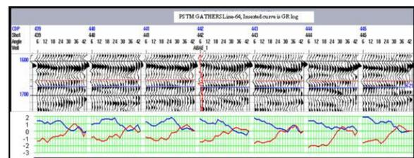
Fig-8 PSTM gathers of line b-b' near well R indicates phase reversal on far offset. Pick values of amplitude along the horizon near sand top (red) and sand bottom (blue) of the gas sand are displayed at the bottom.
