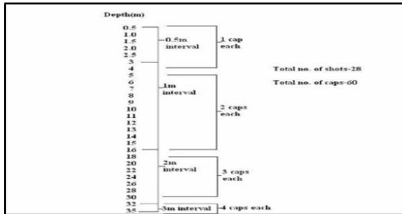
Figure 5: Uphole depth profile and caps / detonator information
