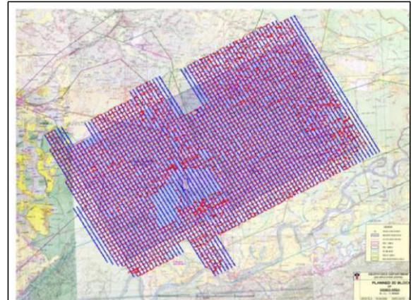
Figure 2: Superimposed actual Source and Receiver Positions of Digboi-Margherita 3D block on Base map
