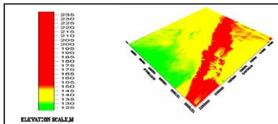
Figure 3: Elevation model for Digboi -Margherita 3D Block; Elevation varies from 125 m to 235 m
