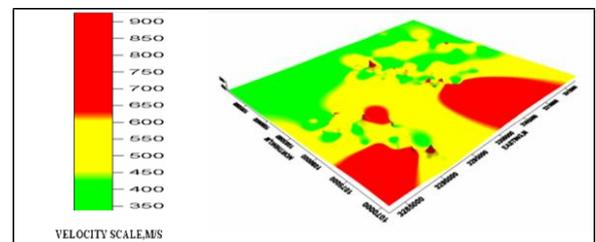
Figure 7: Weathering layer velocity model for the Block; Velocity varies from 350 m/s to 900 m/s
