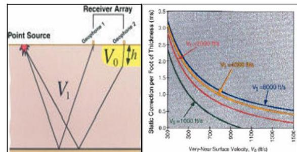
Figure 1: Simple point-source/receiver array model with flat topography (Left), Static correction in ms/ft for various surface alluvial velocities ( $V_0$ ) and various underlying layer velocities ( $V_1$ ) (Right)
