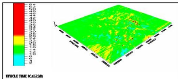
Figure 11: Uphole time model for Digboi - Margherita 3D Block
