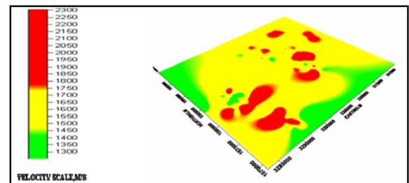
Figure 9: Sub-Weathering layer velocity model for the 3D Block; Velocity varies from 1300m/s to 2300 m/s
