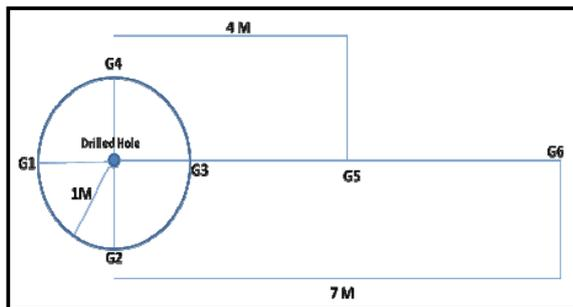
Figure 6: Uphole Spread Geometry & Geophone positions
