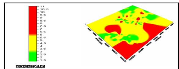
Figure 8: Weathering layer thickness model for the 3D Block; Thickness varies from 1.5 m to 11 m
