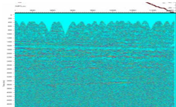
Figure 12: Brute Stack after static correction applied showing the reflectors clearly.
