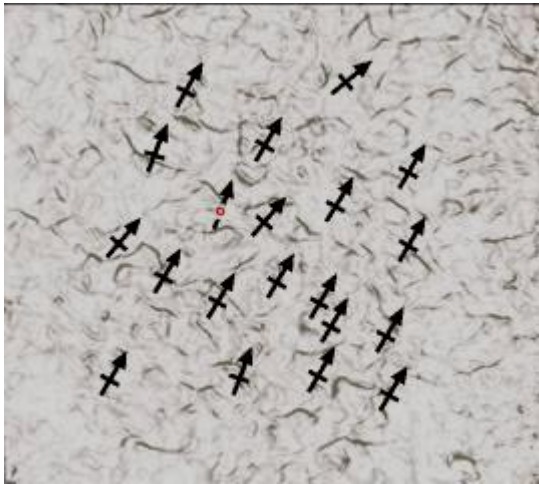
Figure 8: Map showing overlay of \varphi on a discontinuity cube showing fracture network.
