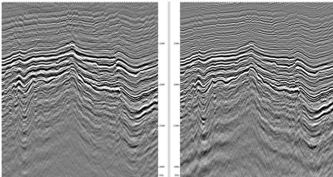
Figure 7: A comparison of Pre STM Stack (left) and PSDM (scaled) from this area showing Improvement in imaging at Basement level
