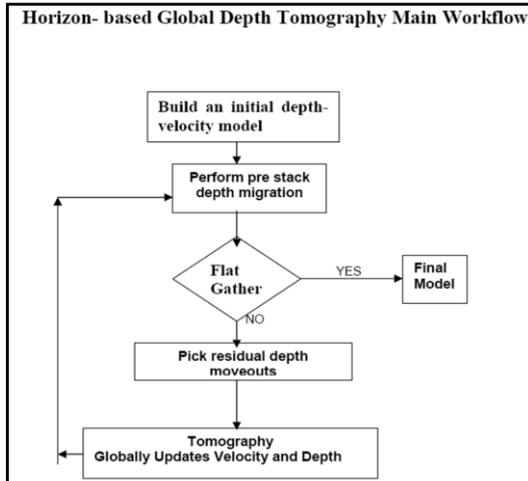
Figure1: shows the flow chart of the PSDM followed for the present project
