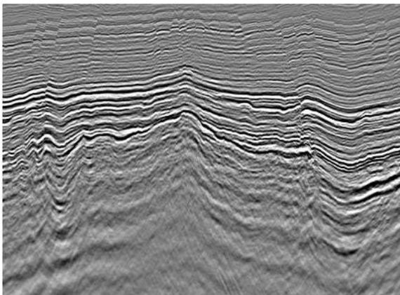
Figure 5(b) PSDM Stack scaled to Time Migrated .shows delineation of fault pattern.
