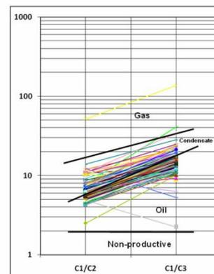
Fig-2: Pixler plot to discriminate oil, condensate and gas zones of study area
