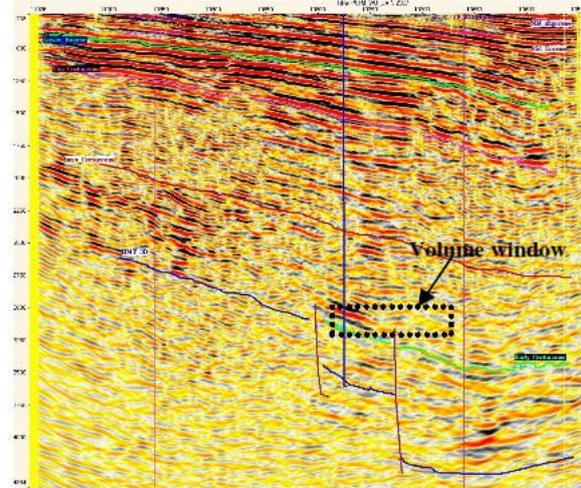
Fig-5b: A seismic section across prospect-C area showing high amplitude reflectors at Top of Early Cretaceous Formation where volume window zone (80 ms) with dotted line.
