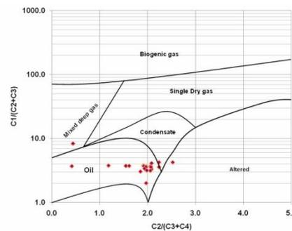
Fig-3: Cross plot between  $C_2/(C_3+C_4)$  and  $C_1/(C_2+C_3)$  for gas signature of study area
