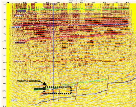
Fig-5a: A seismic section across prospect-A area showing high amplitude reflectors at Early Cretaceous Formation where volume window zone (80 ms) with dotted line.
