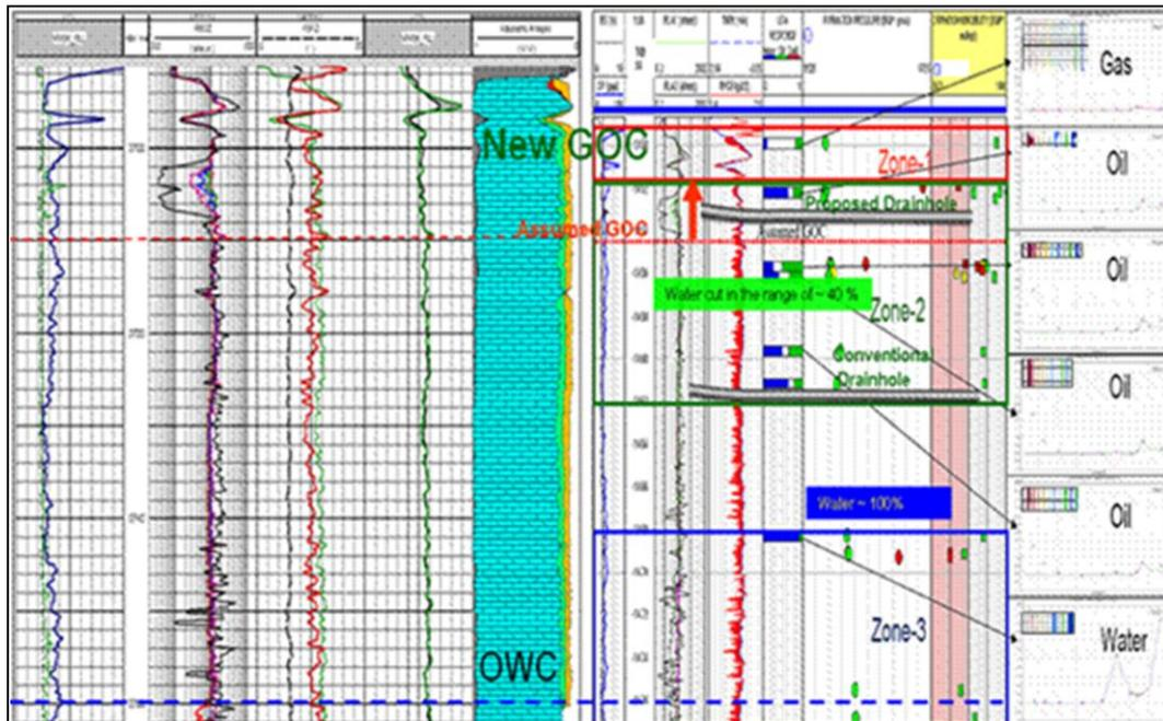
Fig-3 : Well placement using WFT and DFA
