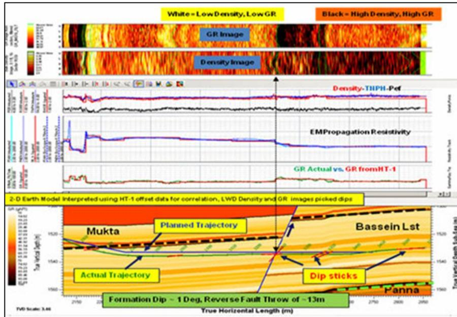
Fig-1 : Well placement across fault.
