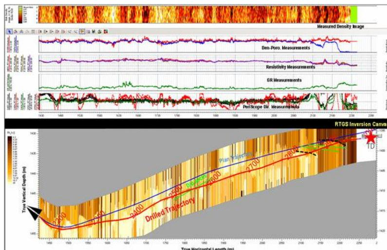
Fig-2 : Well placement using LWD & Imaging of bed boundary
