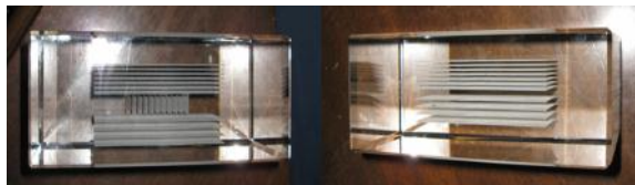
Figure 2. Two other glass models with laser-etched interior fracture zones simulating VTI and HTI regions.
