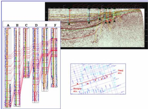
Fig. 4: Calibration of electrolog with seismic passing through Hirapur-Gamij area and correlation of T/R sequence on logs
