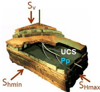
Figure 1: Geomechanical Model comprises in-situ stresses, rock properties and pore pressure.
