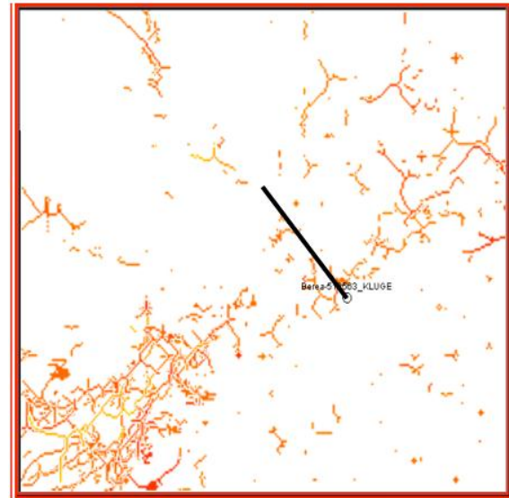
Figure 2: Map slice of the reservoir permeability field activated during one frac stage. The map is a slice at the level of the lateral. Length of lateral = 1 km. Of particular interest
